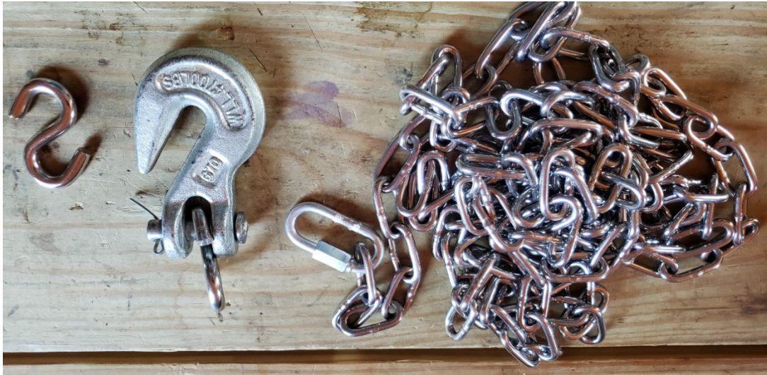
Figure 2. Stainless steel 5/32" (4mm) chain and hooks etc. Load capacity >500lb.
