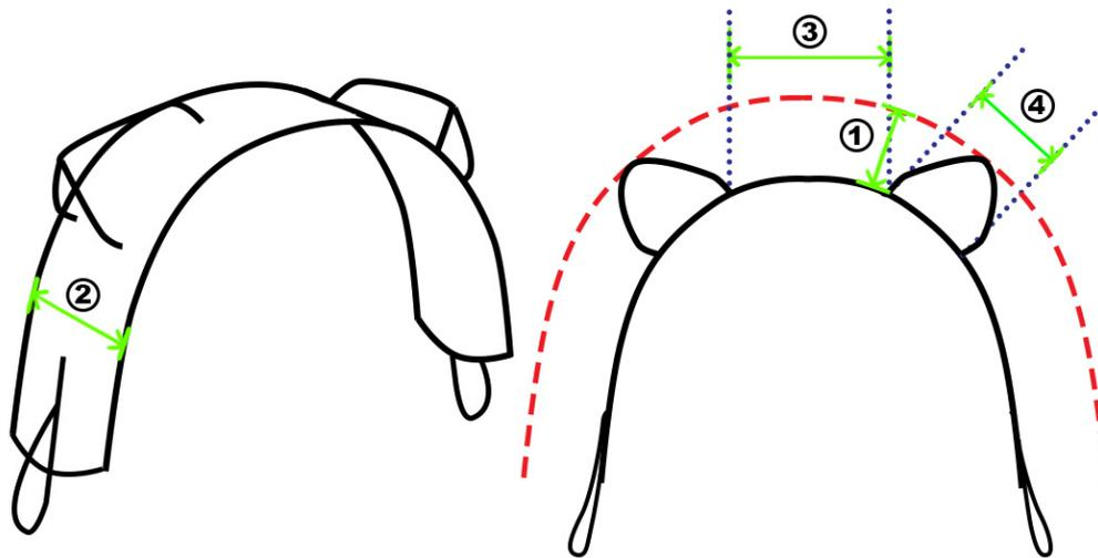
1. Maximum distance measured from flat face of surcingle to outer point of handles 180mm.
