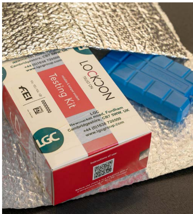
Figure 19 : Testing kits and a freezer pack(s) should be placed into the isothermal bags
