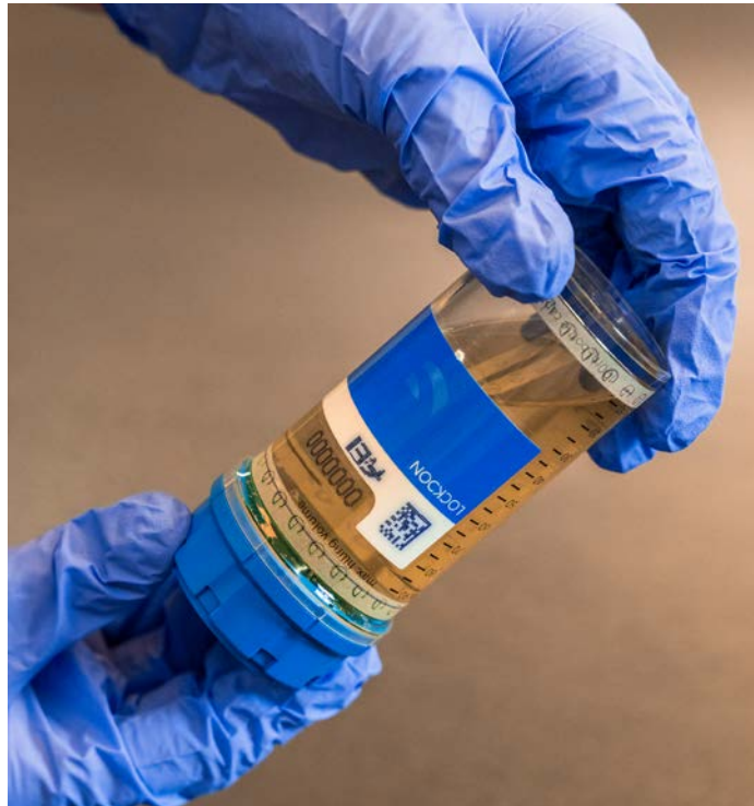
Figure 8: Turn the sealed bottle upside down to ensure there is no leakage
