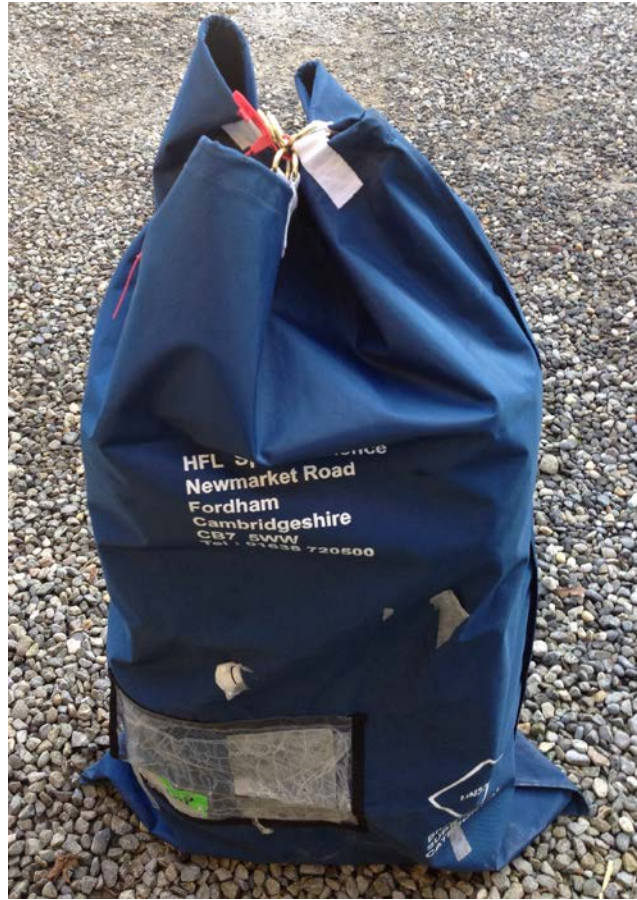
Fig 21: The blue carrying bags should be securely fastened with the red plastic clip
